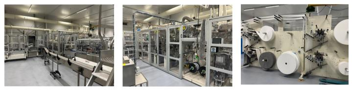
Speed: 600 ppm, size: 175\*95 mm, power supply 120 kW, power consumption 90 kW/hr, effciency >90%, waste <3%, compressed air supply 6 bar, air consumption 2000 NL/min.
